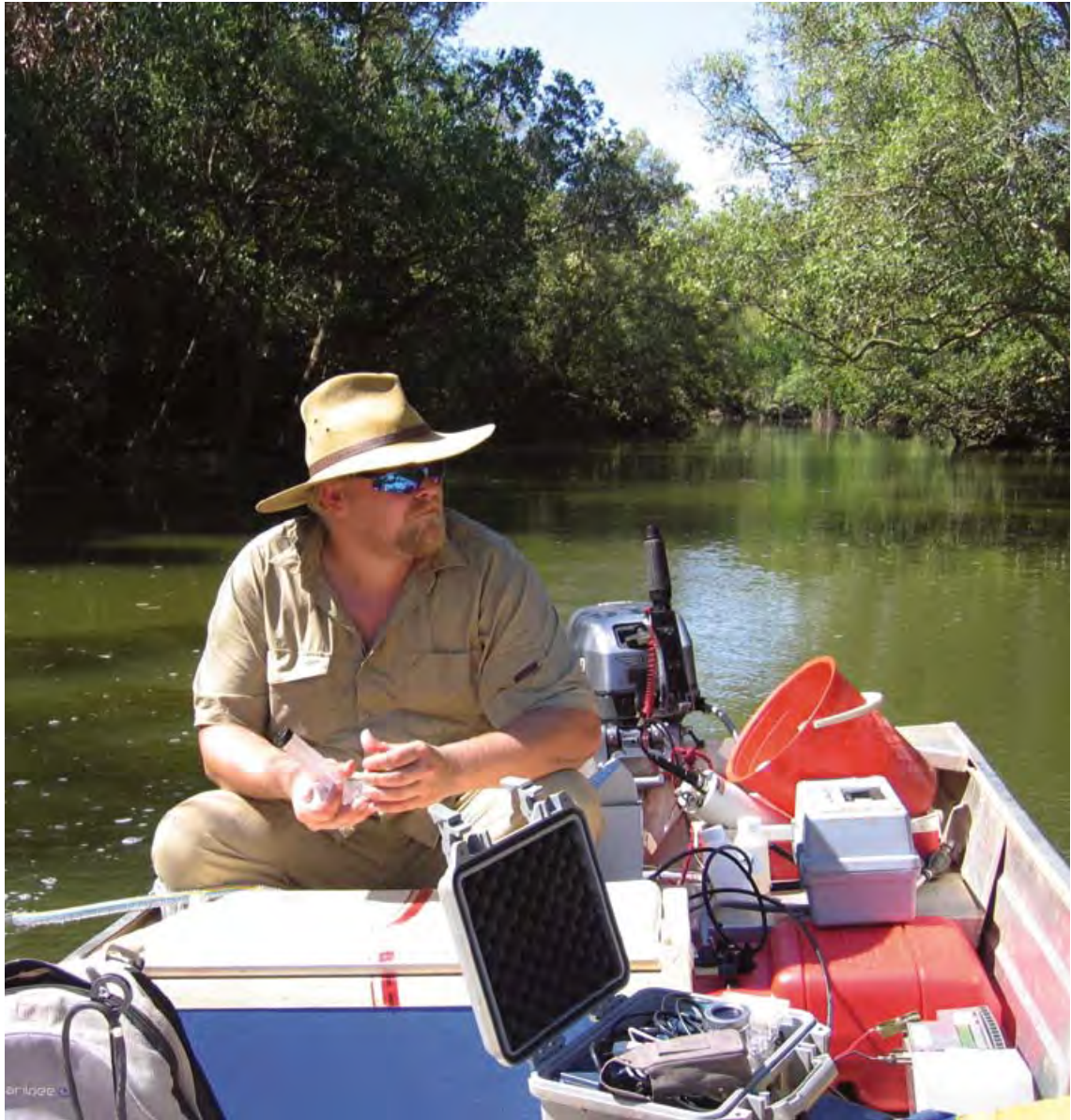
Water quality sampling in Buffalo Creek. Buffalo Creek receives treated wastewater discharge from the Leanyer-Sanderson sewage treatment plant. Water quality is poor, with very high chlorophyll levels – hence the noticeable green colour of the water during this sampling. Photo: Julia Fortune
